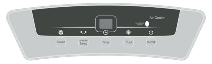
**ON/OFF:** Press once this button to make the unit ready for working. It will start up with MID in 3 seconds and then revert to work under the memorized status. If for first time use, it will start up with MID in 3 seconds and then work with LOW.
